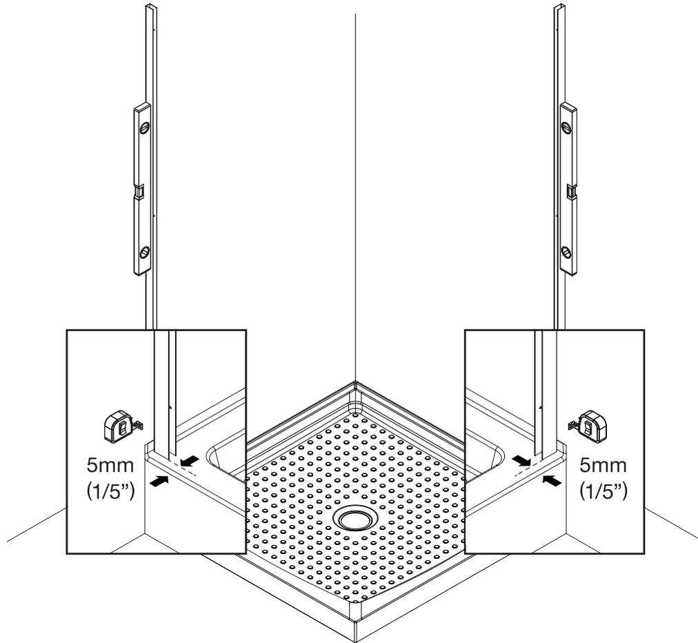
**1.1** Position the wall jamb as the picture, make sure it is vertically, then mark the hole location by pencil.
